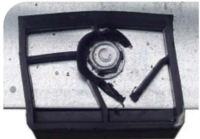
Fig 2: Over driven – cross hairs snapped
