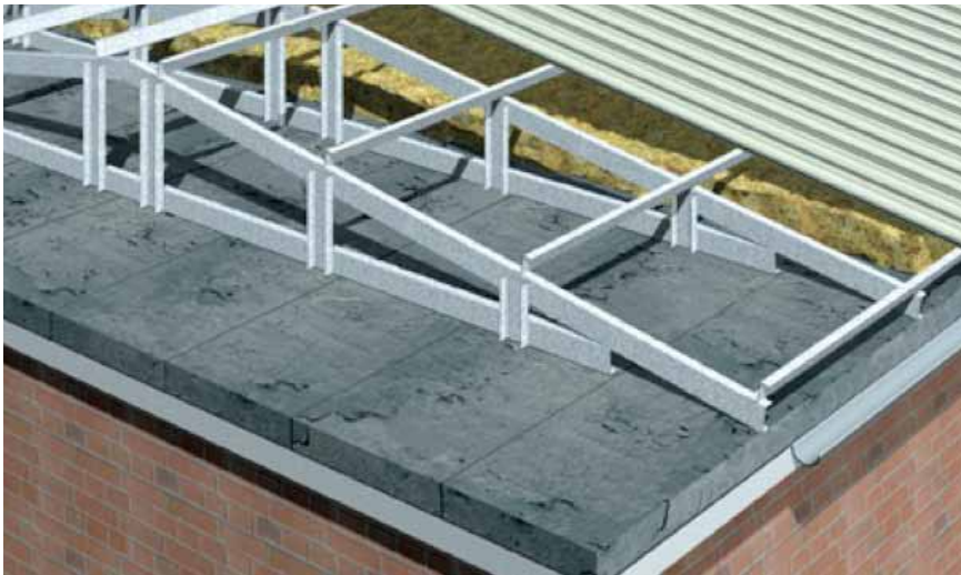
Figure 11. Pre-finished steel pitch framed roof system installed on building with a flat roof
